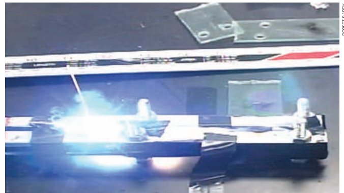
FIG. B IS a picture of my rail gun being fired. The blue spark is a piece of tin foil being vaporized to create plasma.
