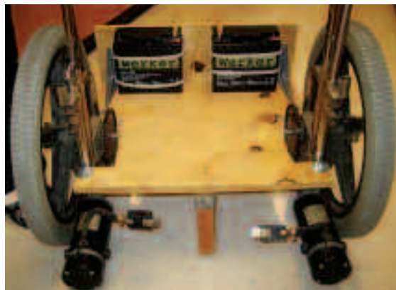
A ROUGH prototype of the Segway the group made.
