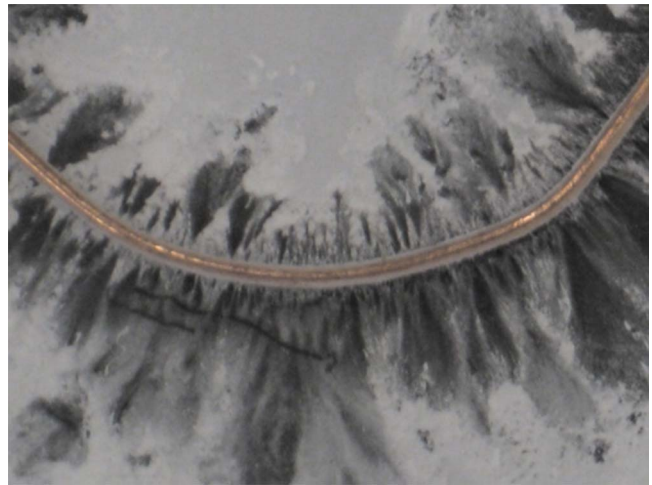
Fig. 2. This is a 400%-magnified version of Fig. 1. It shows the copper wire and the electric field lines close to the wire.
