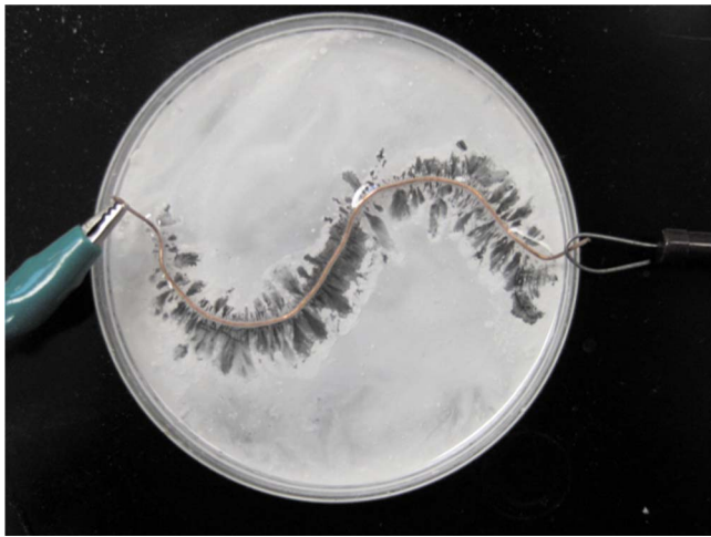
Fig. 1. The picture shows a PTFE sealant mixed with mineral oil in an 88 mm diameter \times 12 mm high plastic Petri dish. An S-shaped 1 mm diameter (18 gauge), 13 cm long copper wire is placed in the Petri dish and connected in series with an 8 M \Omega resistor to the power supply (not shown in the picture). The PTFE groups into strands and clumps, which visibly align perpendicular to the wire.
